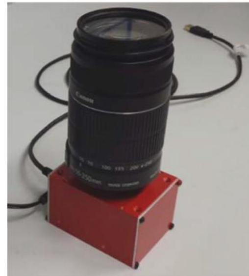
Fig. 1: SPAD camera for 2D imaging, 3D ranging and TCSPC photon-counting.
