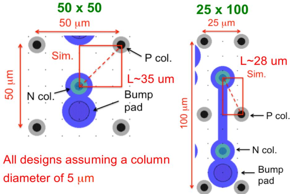
All designs assuming a column diameter of 5  $\mu\text{m}$
