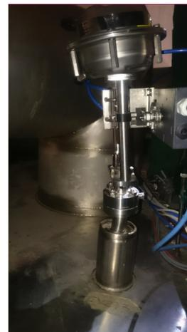
Severe mechanical damage, consistent with large forces applied near base then opposite force applied to pneumatic driver.
