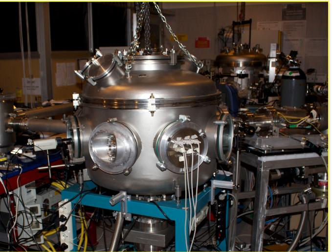
A separate target chamber is dedicated to laser-gas interaction for:
