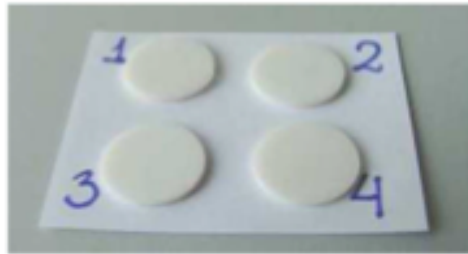
Fig. 8. Visible image of sample with four pellets containing different chemicals: (1) lactose, (2) aspirin, (3) sucrose, and (4) tartaric acid.
