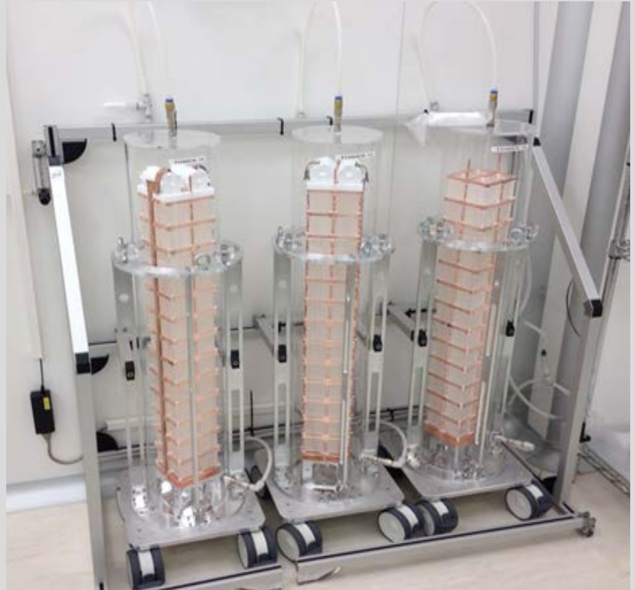
CUORE Towers ready to be installed
