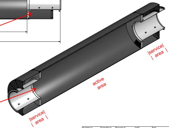
Inner Cylinder made of 20 µm Mylar tube containing the target
