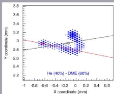
Reconstruction of a real photoelectron track
