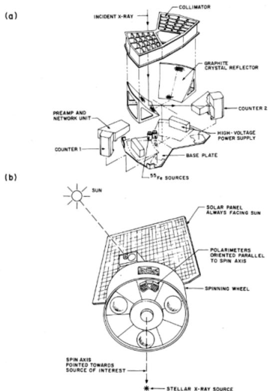
FIG. 1.—(a) Exploded view of the OSO-8 polarimeter assemblies. (b) Location of the polarimeters in the satellite.
