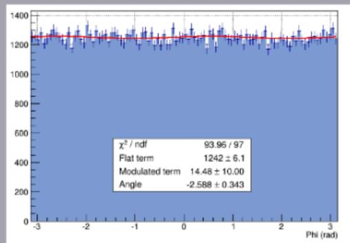
Residual modulation for unpolarised photons
