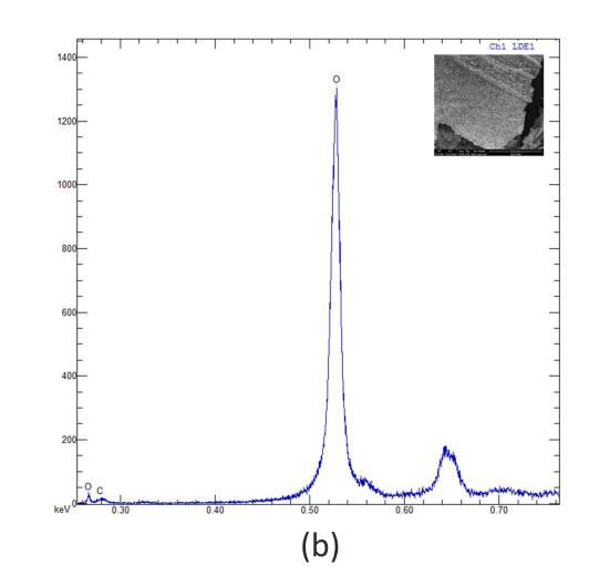
WDS analysis of (a) Few layers Graphene (b) Graphite Oxide
