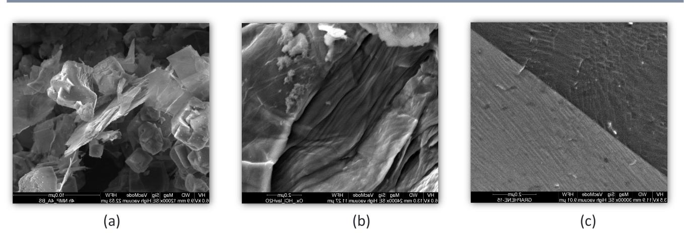
SEM images of carbon-based nanostructures, (a) Few Layers Graphene
