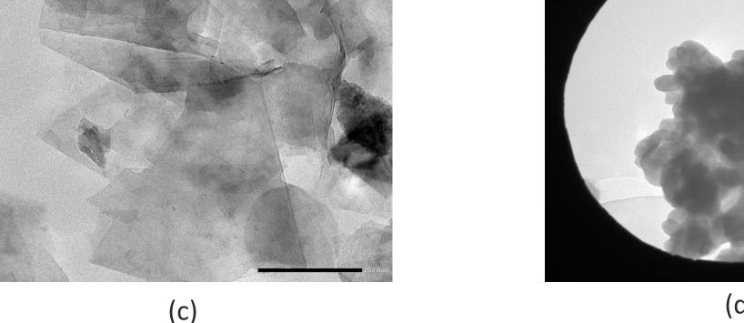
• TEM images of carbon nanostructures, (a) Diffration pattern of Few Layers Graphene; (b) Diffraction pattern of Graphite Oxide (c) Few layers graphene (d) Defined area to make diffraction pattern of GO
