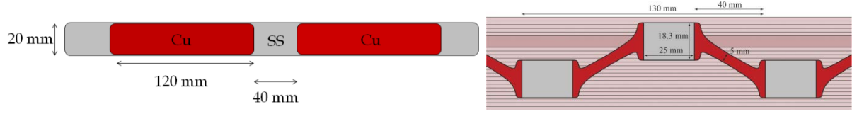
Figure 3-5: Sketch of quench heaters for the outer layer (left) and a design for the inner layer (right); stainless steel (SS) in grey and copper cladding in red
