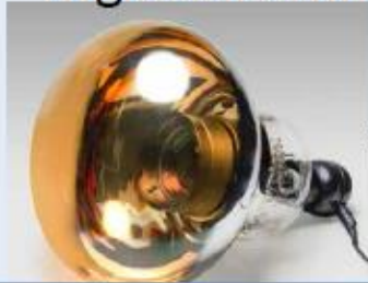
Venetian blind PMT (50-cm \phi Normal QE)
