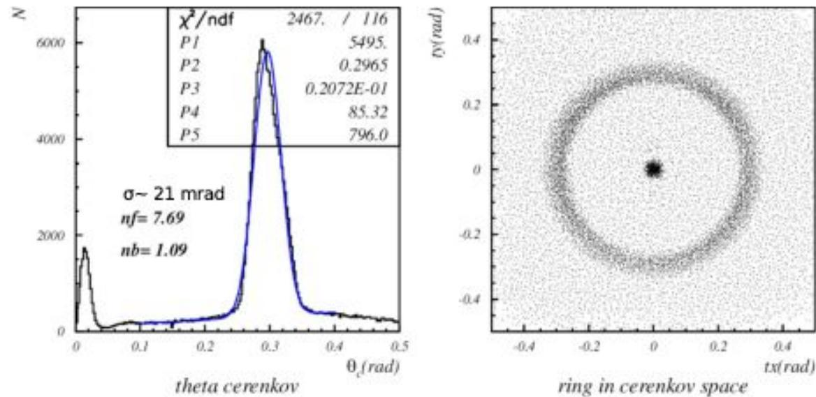
Two 2cm aerogel layers in focusing configuration
