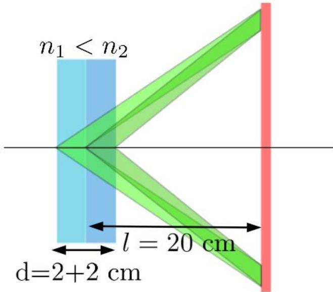
Two aerogel layers in focusing configuration:
