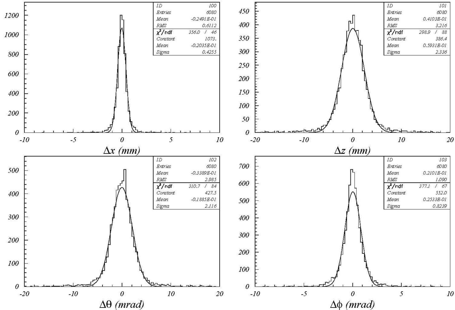
Expected resolutions for a TOP module positioned at  $r = 165$  cm
