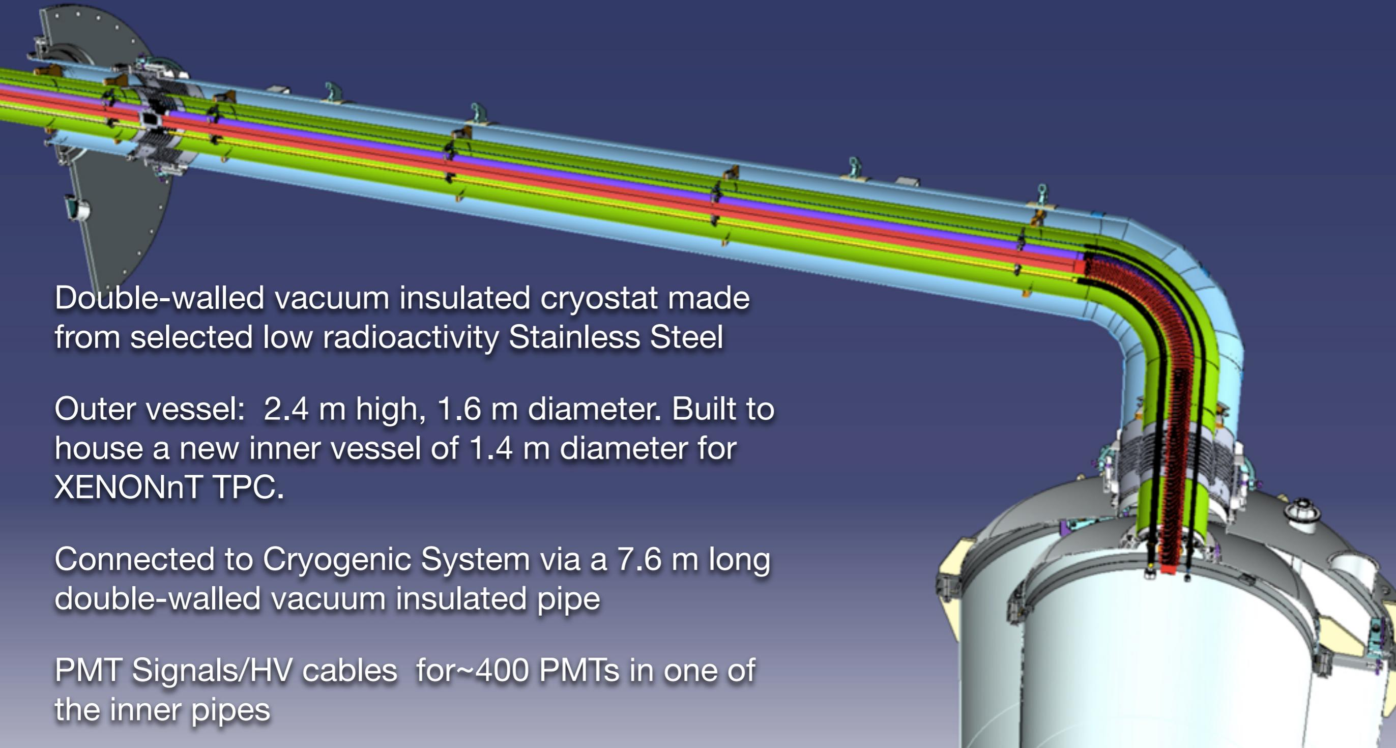
Double-walled vacuum insulated cryostat made from selected low radioactivity Stainless Steel
