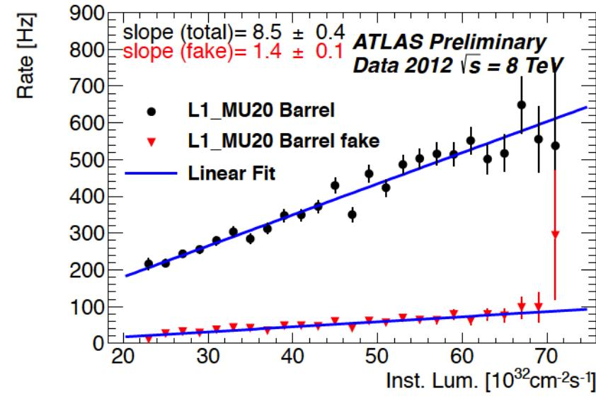
Rate scales linearly with luminosity in the measured range
