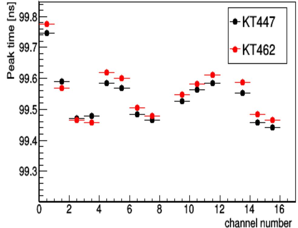
Channel-by-channel differences are due to differences in the cabling lengths for each channel; PMT-PMT offset due to different fiber positions
