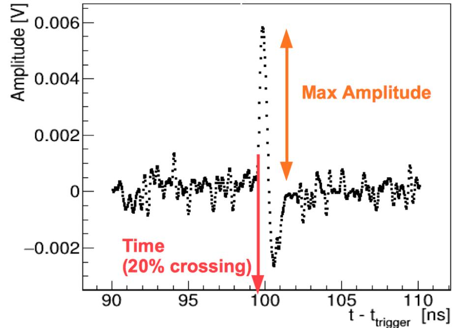
Typical signal pulse (inverted)
