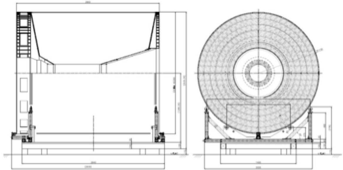
Figure 2: Two-dimensional CAD drawings of the CDC on top of the support stand in the Tsukuba Hall alcove (provided by Kohriki-san).
