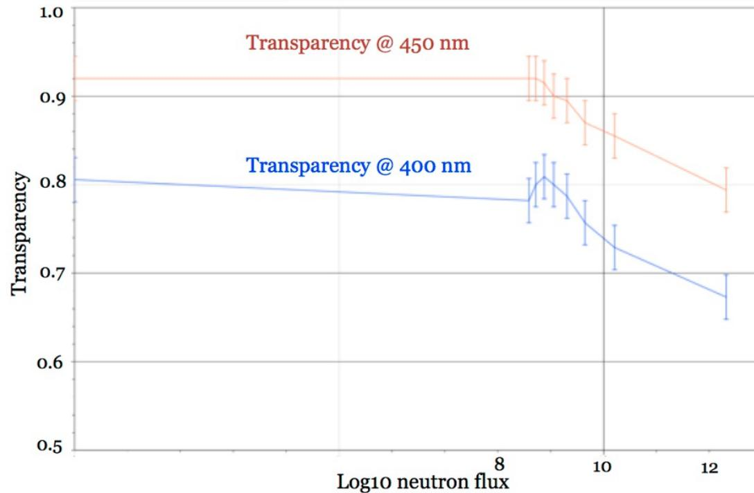
Irradiation of 9 GRIN lenses at variable distance from the target
