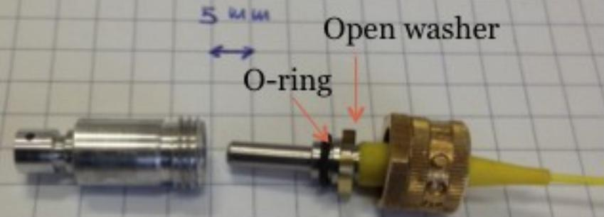
Connections between fibers, grin lens and iTOP prism designed by the PD mechanical workshop
