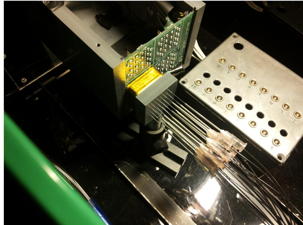
16-channel readout with CAEN V1742 switched capacitor digitizer almost ready
