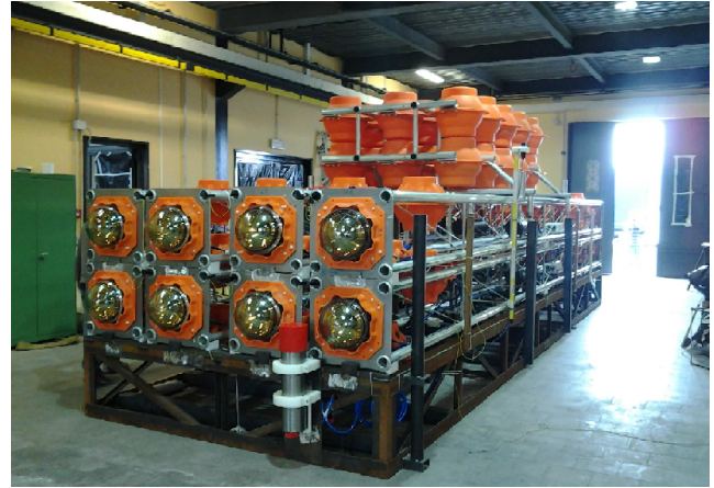
Fig. 4 The tower in compact configuration during the integration phase.
