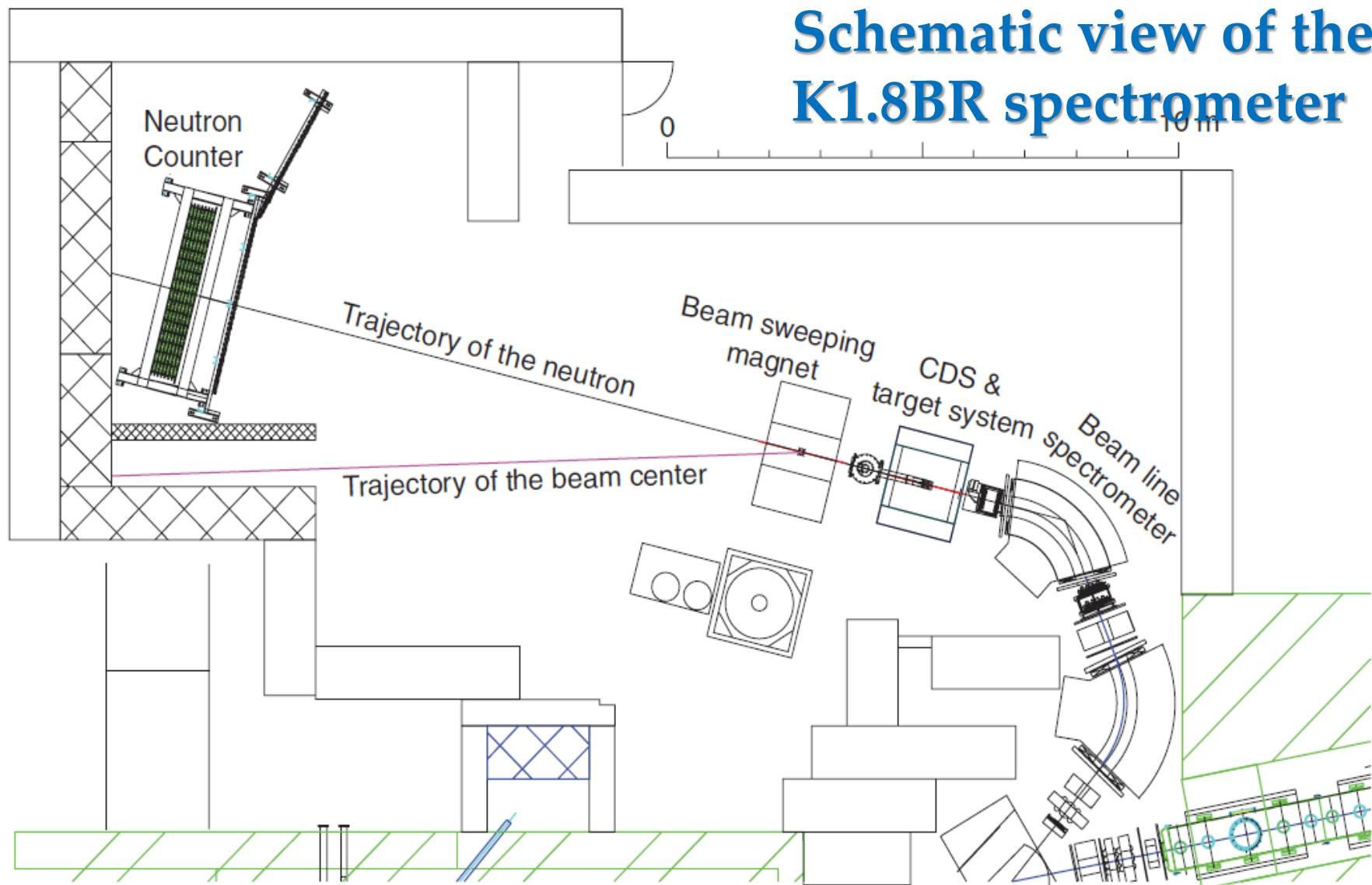
The spectrometer consists of a beam line spectrometer, a cylindrical detector system that surrounds the liquid  ${}^3\text{He}/{}^4\text{He}/\text{D}_2$  target system to detect the decay particles from the target region, a beam sweeping magnet, and a neutron time-of-flight counter located  $\sim 15\text{m}$  downstream from the target position.
