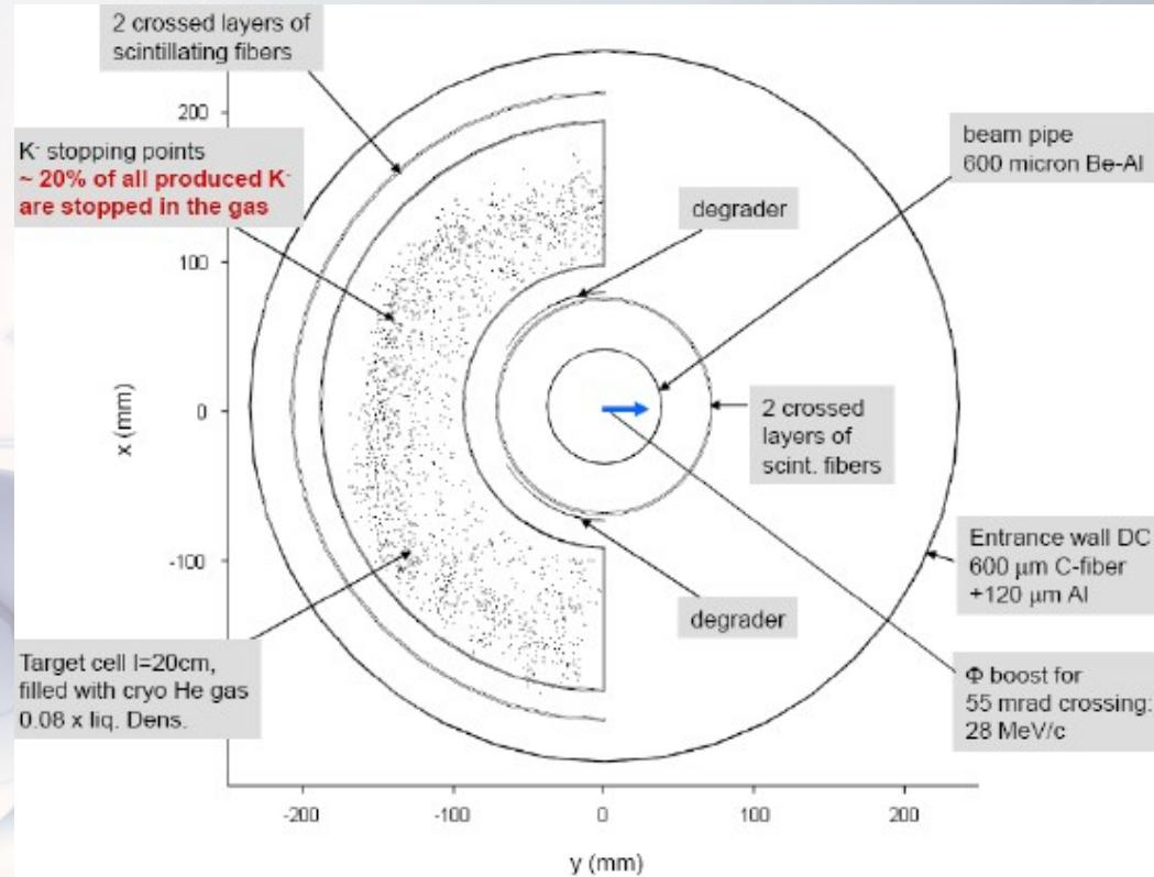
Possible solution for a half-toroidal cryogenic target cell, inside a vacuum chamber, and two more layers of fibers.
