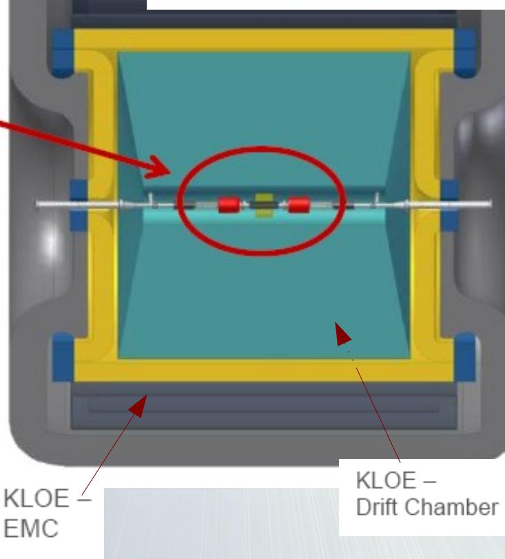
**•Target** (A gaseous He target for a first phase of study)
