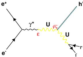
**Figure 4.** Dark Higgsstrahlung process in the *invisible scenario* with a long lived dark higgs  $h'$  which escapes detection producing a missing energy signal ( $l = e, \mu, \pi$ )
