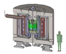
**Figure 5.** The proposed setup for the J-PARC g-2 Experiment. Muons enter at the top left (green trajectory) and spiral into the highly uniform magnetic field region. Their decay positrons curl inward to an array of silicon tracking detectors. Figure courtesy T. Mibe.
