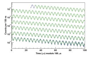
**Figure 2.** E821 anomalous precession data, including fit. The data is wrapped around every  $100\,\mu s$ . Figure courtesy E821 collaboration.
