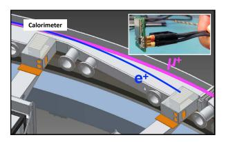
**Figure 4.** Positioning of two of the segmented calorimeter stations just downstream of the scalloped section of the vacuum chambers. The central muon orbit is sketched in, as is a nominal decay positron. The inset shows the size of the SiPM readout and its custom amplifier and pulse-shaping board.
