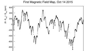
**Figure 3.** First "as built" raw field map for the reassembled storage ring magnet for E989. The nominal field is 1.4513 T. The lumpy features will be greatly reduced as the shimming process begins (see text).
