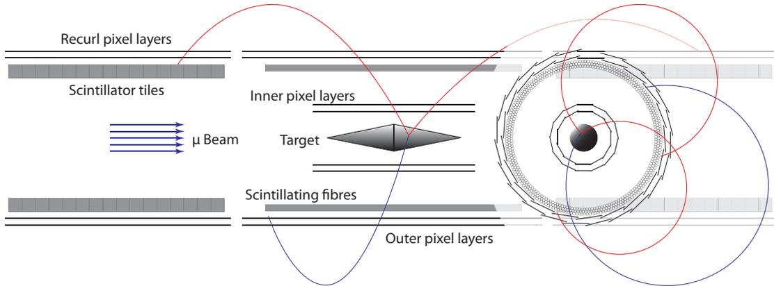
**Figure 4.** Schematic layout of the Mu3e detector in phase IB to be operated at  $10^8$  muons/s.
