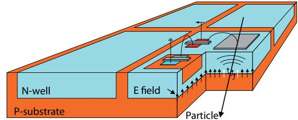
**Figure 5.** Schematic of a pixel sensor in HV-MAPS technology. Taken from [9].
