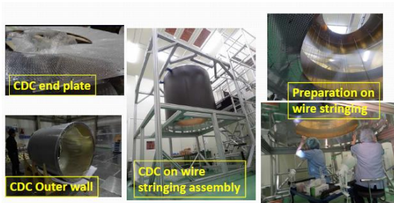
Figure 15. Construction of the CYDET detector
