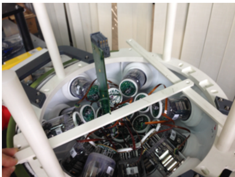
Connection of the PMT tails to large Octopus board
