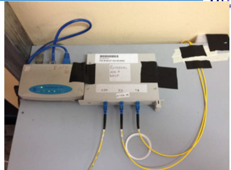
The external add & drop connecting the CLB to the PC
