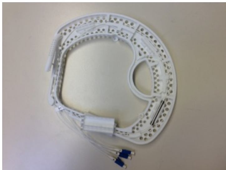
Add & Drop filter routed into the fiber tray
