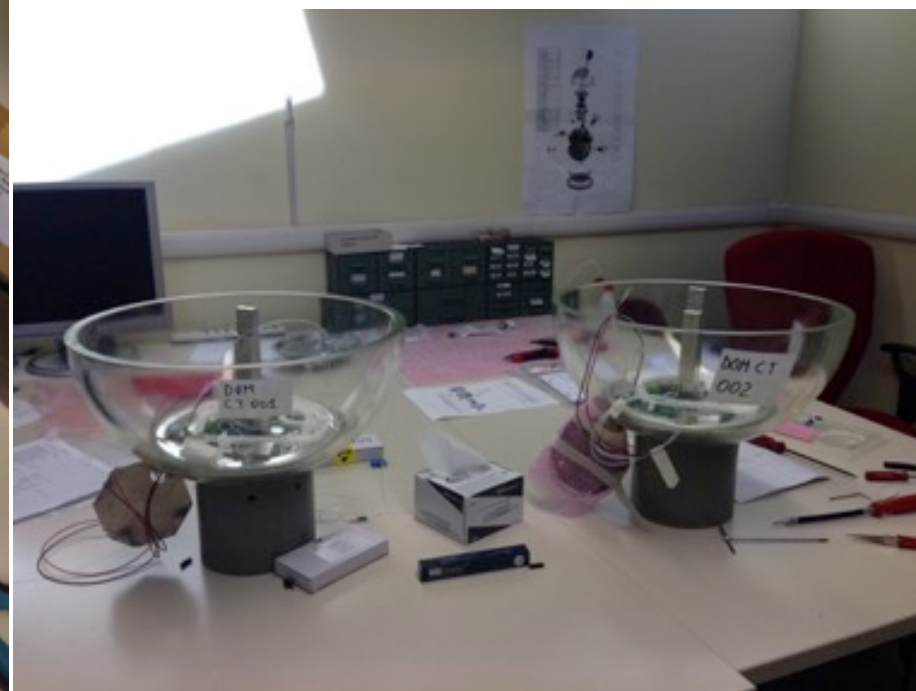
The two prepared top hemispheres: electronics, SFP, add & drop and splice done
