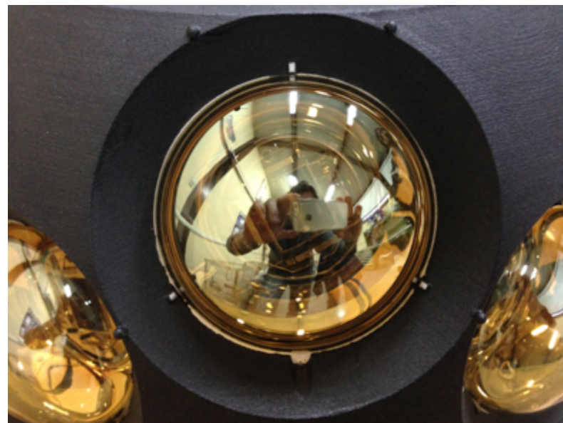
Installing of the PMT respecting tails orientation
