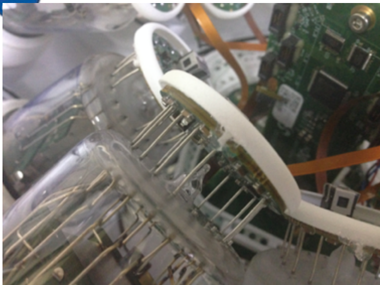
Mounting of the HV fence even by a drop of glue
