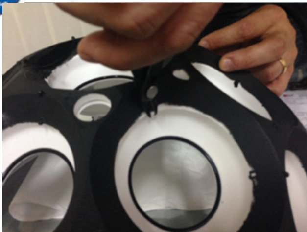
Cutting of the pins for the PMTs
