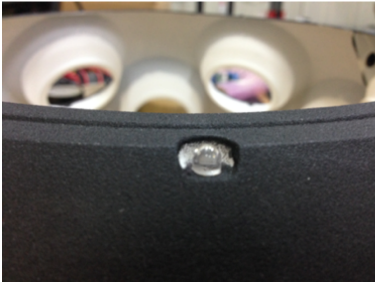
The nano beacon externally levelled with the structure
