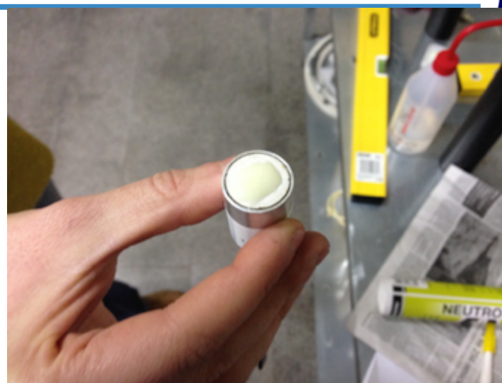
Few drops of glue on the piezo surface
