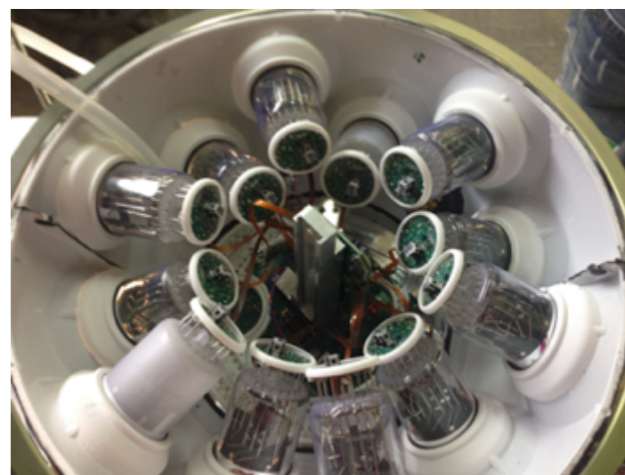
Connection of PMTs to the small Octopus board
