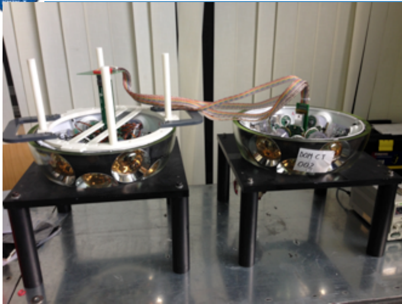
Leiden cable connecting large Oct. Board to CLB
