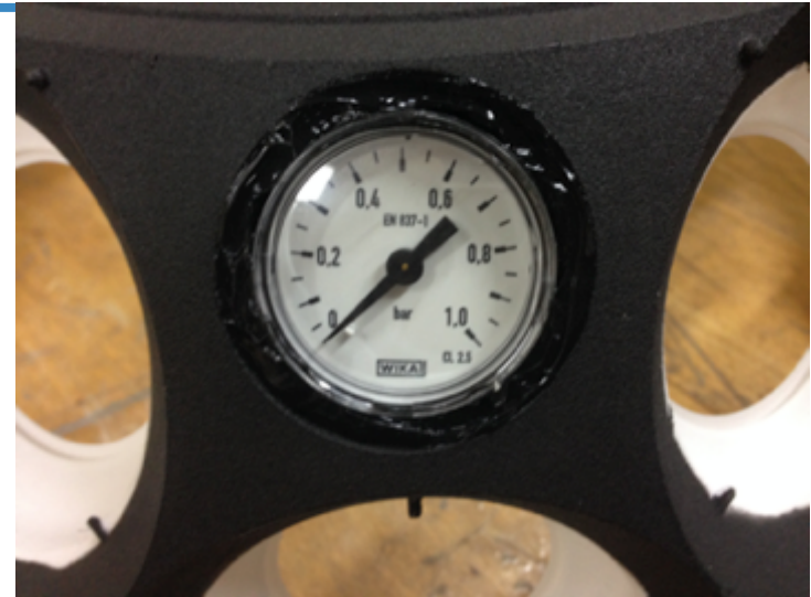
The manometer after the silicone drying and the removing of the tape
