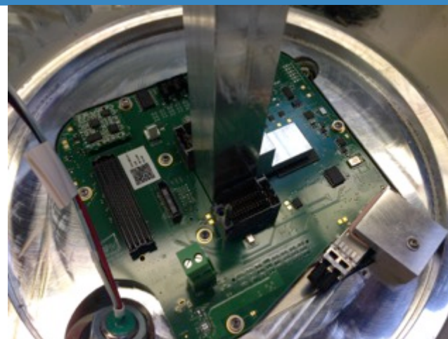
SFP transceiver and cooling blocks
