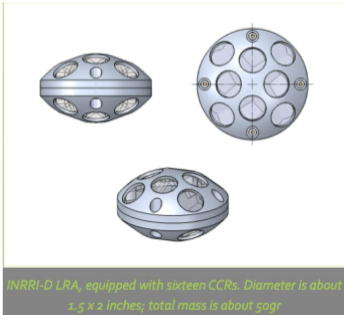
*INRRI-D LRA, equipped with sixteen CCRs. Diameter is about 1.5 x 2 inches; total mass is about 50gr*
