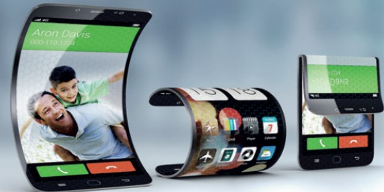
Figure 1 | Graphene-based multi-touch screen showing excellent flexibility (left) 7 and possible applications in bendable or foldable mobile devices (right)
