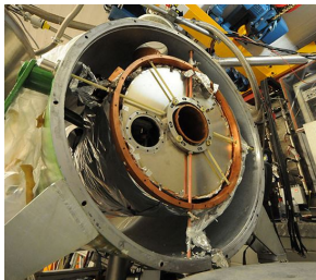
Figure: SERSE was the most performant ion source until the beginning of 2000s
