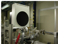
Figure 2. The high temperature L'Aquila-Camerino glass furnace for combined x-ray absorption and diffraction (custom version installed at XAFS@ELETTRA) and the vertical configuration for MAR image-plate detector.
