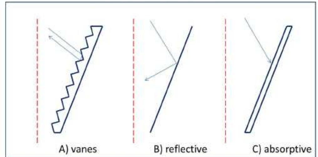
**Absorptive inner sheet:** 10mm thickness /  $n = 1.82$  /  $\tan \text{ loss} = 0.057$
