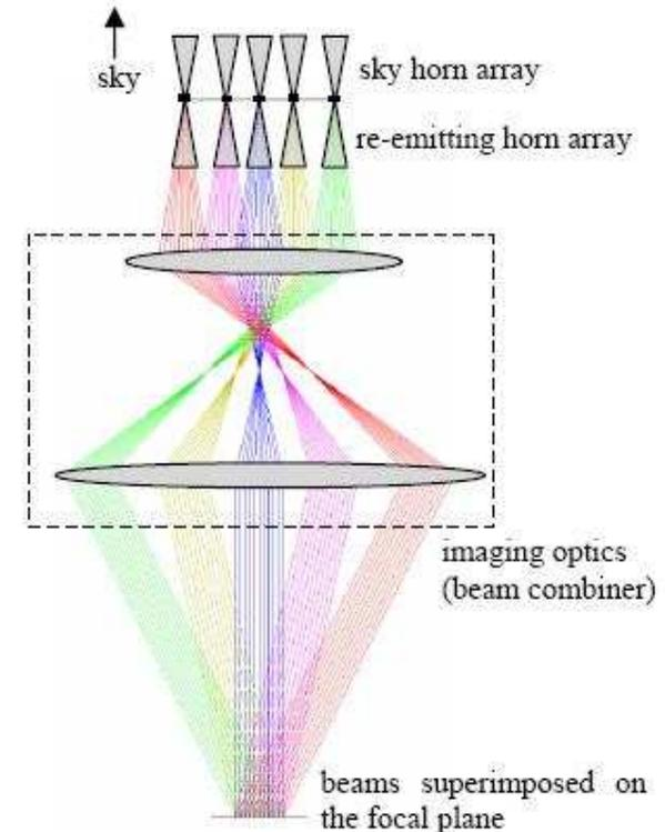
✓ QUBIC operates as an adding interferometer : Fizeau approach
