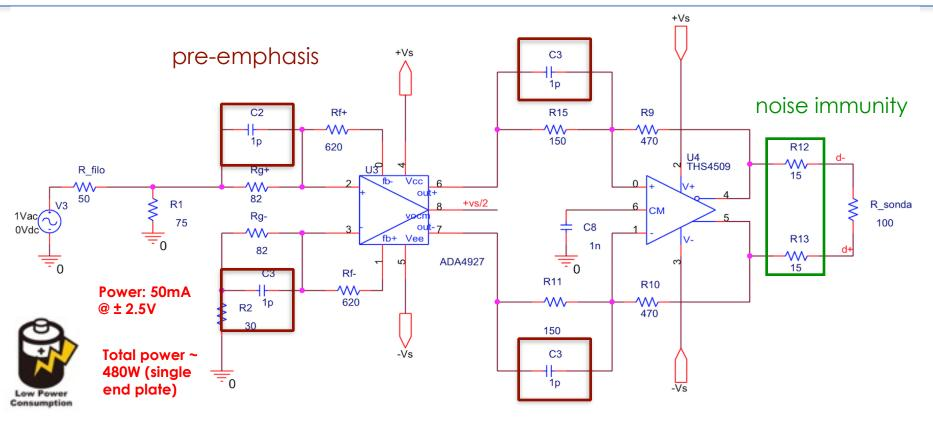
The input network provides decoupling and protection, signal amplification is realized with a double gain stage.
