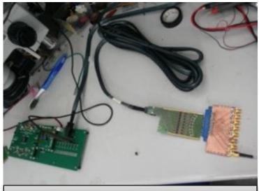
A power supply board based on the same ICs (LTM4614EV, LTM8022V) used on the WD board to power the FE has built The board host a receiver (differential to SE) to test cables/FE cards
