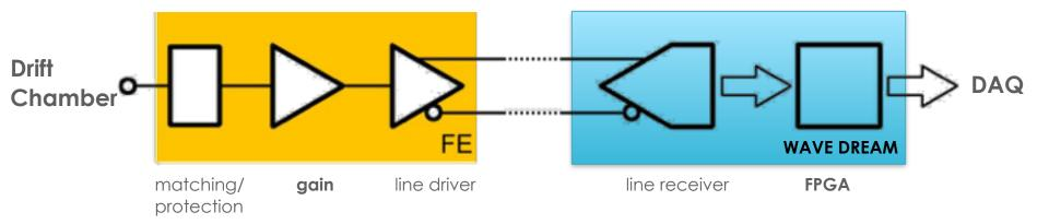
In order to amplify signal coming from Drift Chamber a multistage, low noise and low distortion Front End was designed that provides a total voltage gain of the order of 10 with a suitable bandwidth. Finally signals will be digitized by the MEG Wave Dream digitizer developed at PSI
