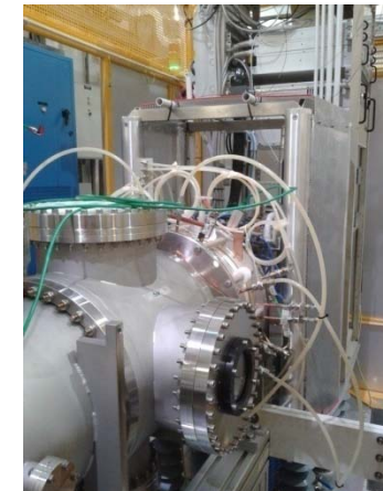
Some water cooling loops for extraction grid EG
