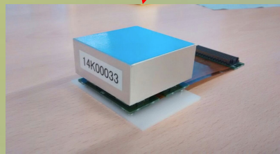
Detection module, 51.2 x 51.2 mm 2 cross section
