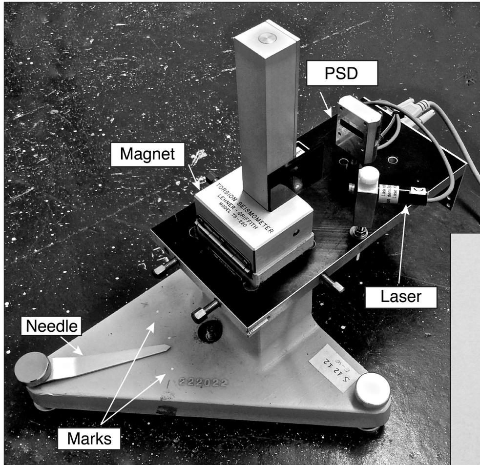
▲ Figure 2. (a) Top view and (b) side view of the Wood–Anderson seismometer currently operating in Trieste. The screws for tuning the beam position, the period and the damping factor, and for blocking the mass of the instrument are shown in the side view.
