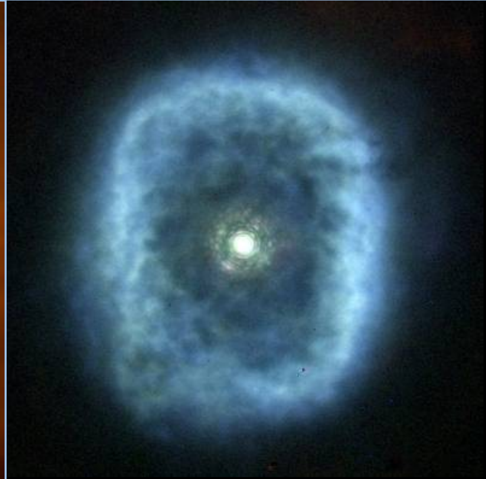
LBT AO, 100s, H2 filter (2.1 \mu m), ref. star Rband 11mag, 150modes, 500Hz
