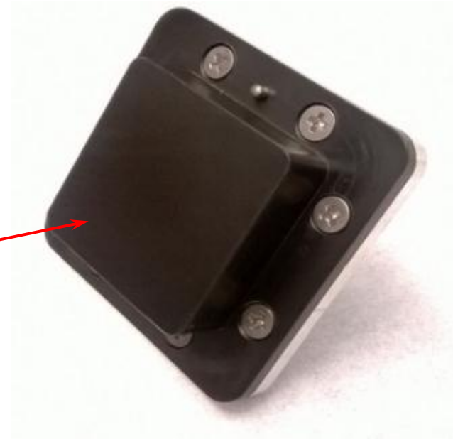
soldering ball transfer tool in conductive material (Tecaform)
