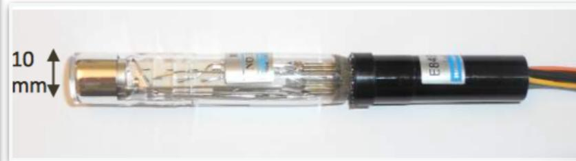
Vecchi PMT:  $\Phi = 15$  mm
