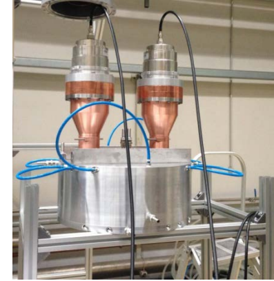
High power RF Coupler 200kW 100% duty cycle
