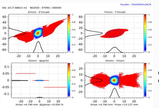
Using a slit size equal to the 94 % of maximum beam size the particles loss are 1 %
