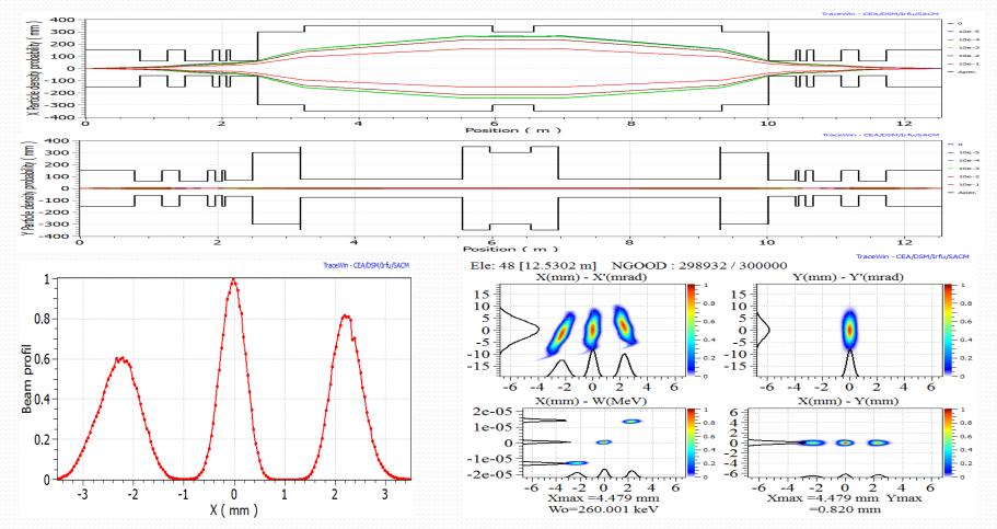
Transverse Gaussian distribution in the phase spaces, truncated at 3, while uniform in the longitudinal phase space with a 1 ev energy spread
