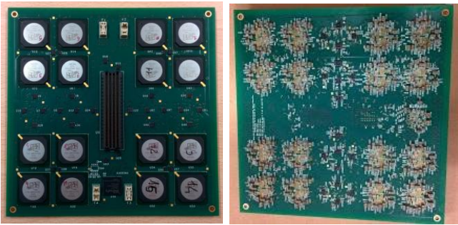
Figure 4. The LAMB assembled with 16 AM chips.
