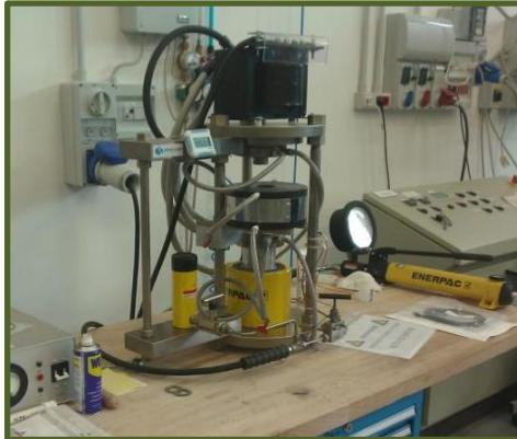
Non end-load Piston-cylinder Press,
