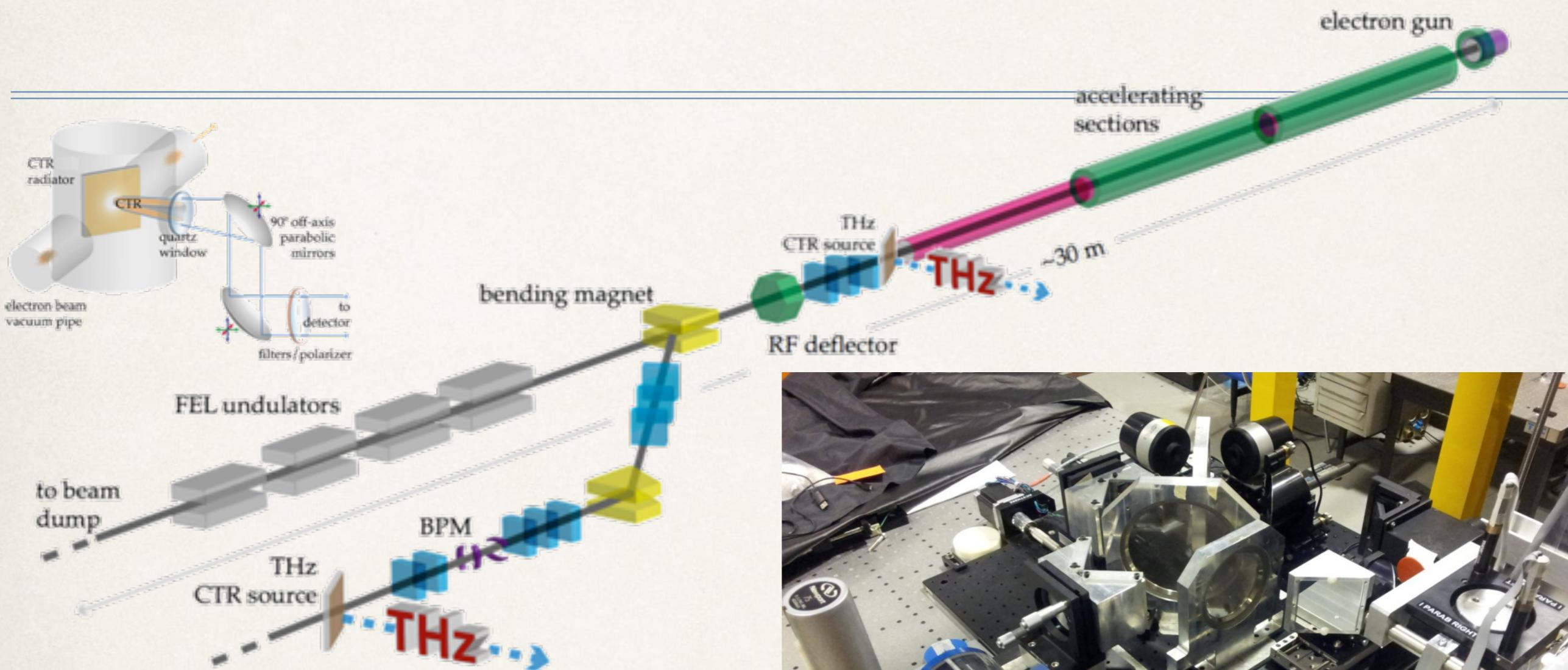
Two stations are dedicated to THz applications and electron beam longitudinal diagnostics by measuring the autocorrelation function of CR through either Martin-Puplett or Michelson interferometer
