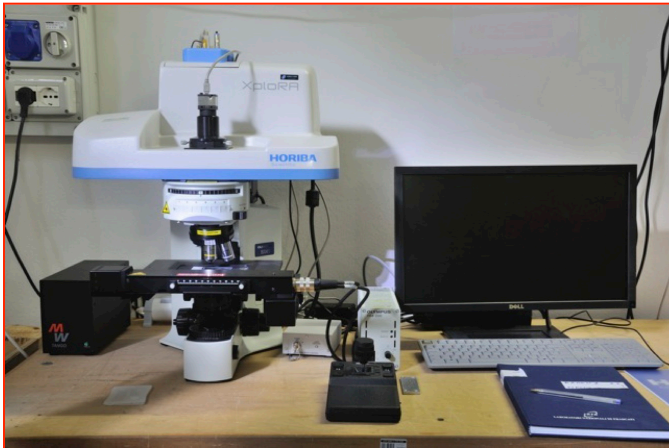
Micro-Raman instrument XPLORA from Horiba Jobin-Yvon (LNF-CSN5)
