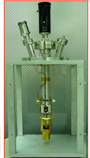
Scanning tunneling microscope (STM) from RHK (LNF-CSN5)
