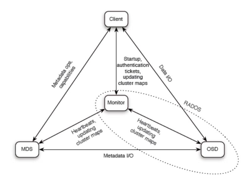
Ceph Clients and Ceph OSDs both use the CRUSH map and the CRUSH algorithm.
