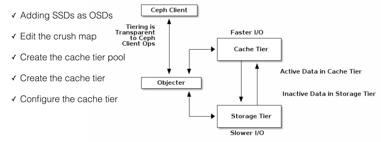
Important note: Once we enabled the cache tiering, Ceph clients with kernel 3.13 stopped working with 'feature set mismatch' error —> kernel upgrade was needed.
