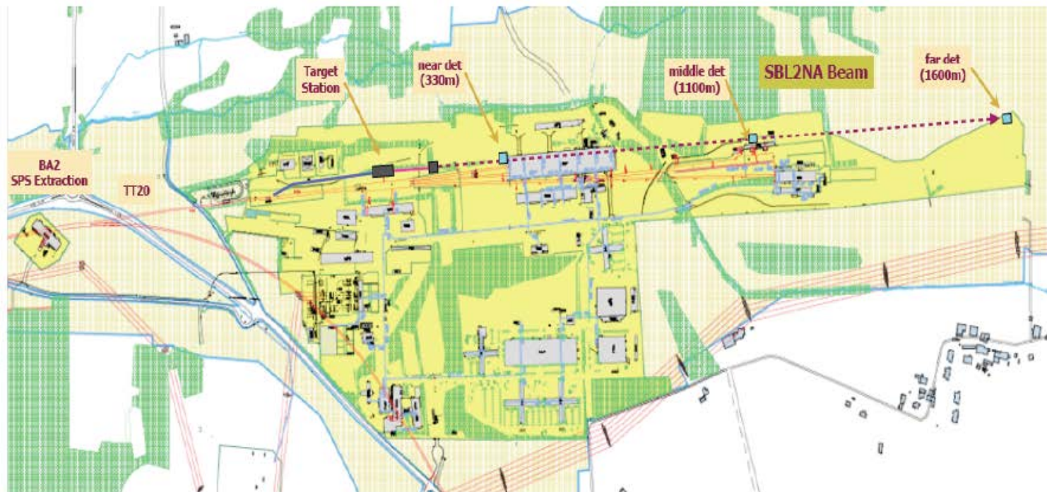
Figure 1: The new SPS North Area neutrino beam layout. Main parameters are: primary beam: 100 GeV; fast extracted from SPS; target station next to TCC2, ~11 m underground; decay pipe: 100 m, 3 m diameter; beam dump : 15 m of Fe with graphite core, followed by muon stations; neutrino beam angle: pointing upwards; at ~3 m in the far detector ~5 mrad slope.
