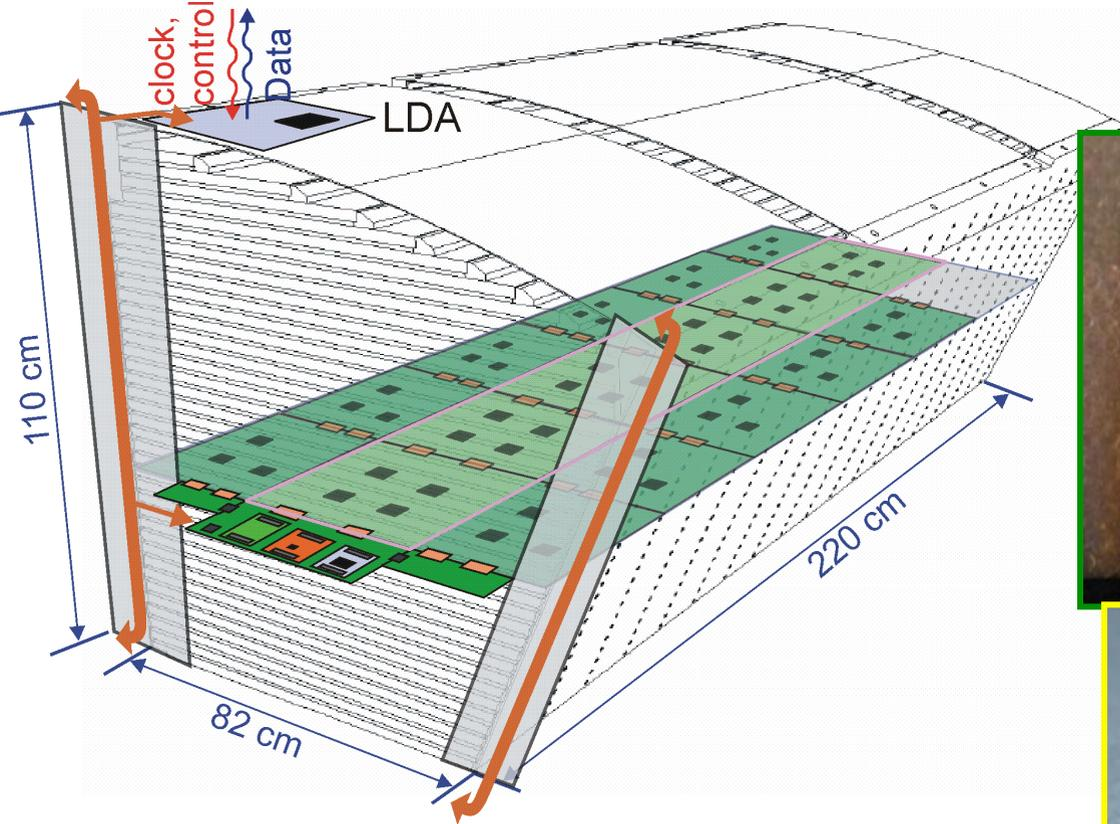
~ 1,000 calorimeter cells / m<sup>2</sup>
