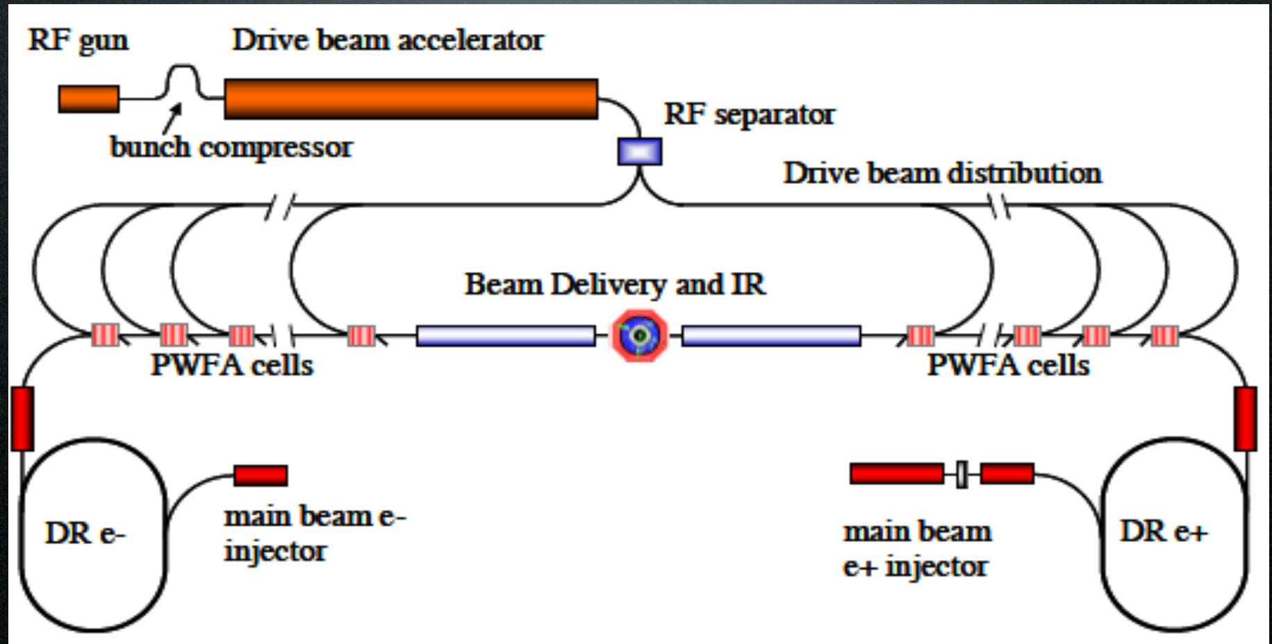
Fig. 1: Concept for a multi-stage PWFA Linear Collider.
