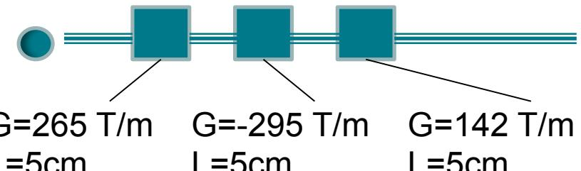
Keeping the **beam size under control** is possible, but **normalized emittance grows** throughout the beamline.
