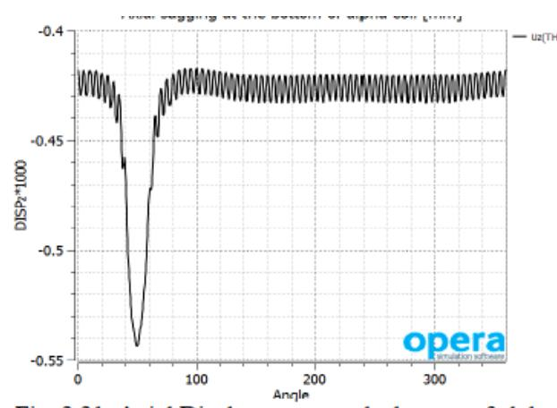
Fig. 2.31. Axial Displacements at the bottom of alpha coil
