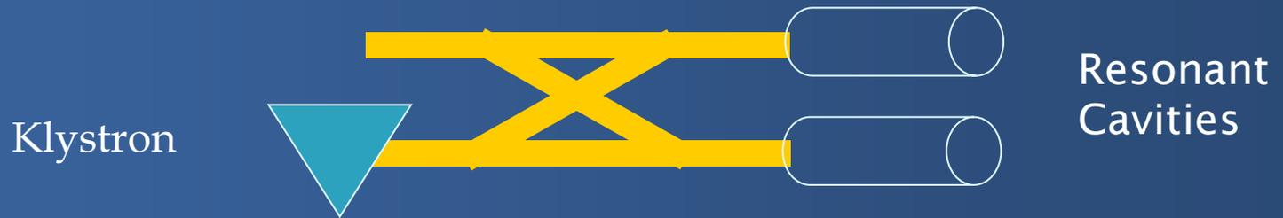
Power from port 1 will be split and flow equally to ports 2 and 3, but with a phase shift.
