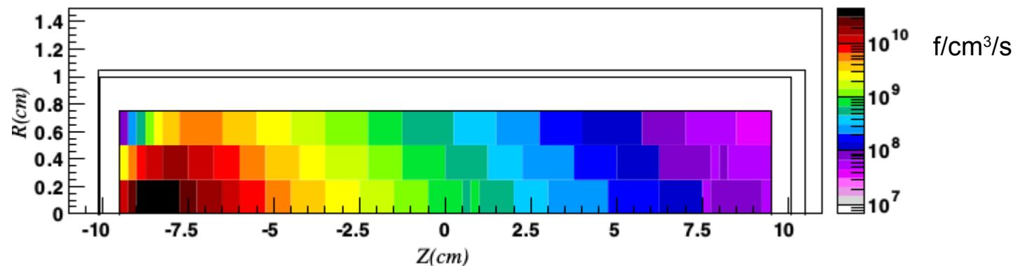
Fluka fission rate in  $3.2 \text{ g/cm}^3 \text{ UC}_x$  target
