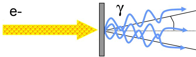
$10 \mu\text{A} \times 50 \text{ MeV } e^- = 500 \text{ W}$  at Alto vs  $1 \mu\text{A} \times 26 \text{ MeV d} = 26 \text{ W}$  at Parrne
