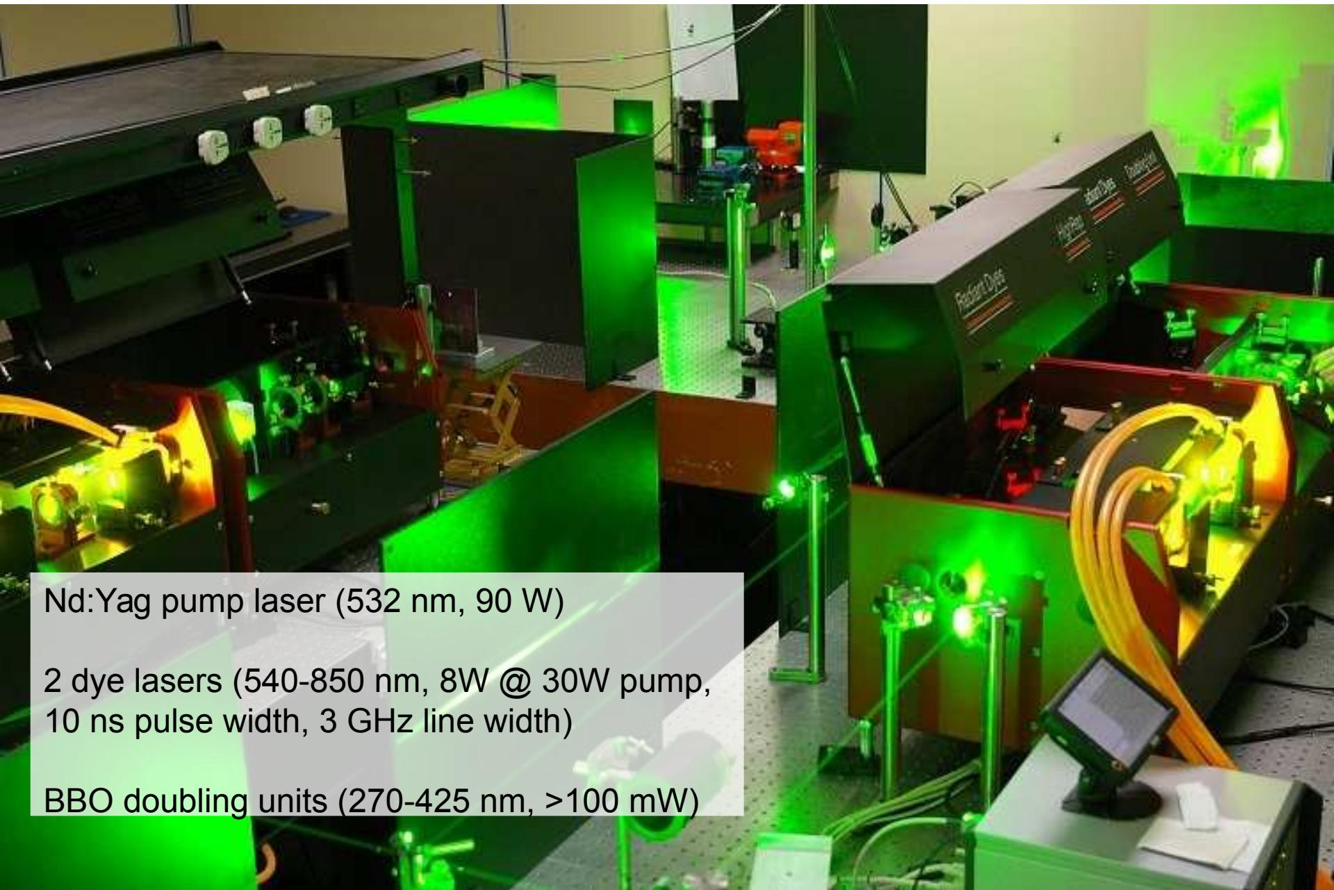
Nd:Yag pump laser (532 nm, 90 W)
