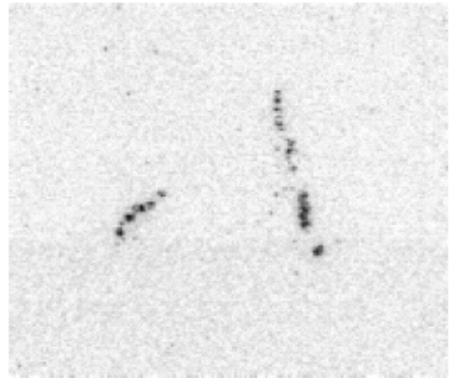
Figure 3. Raw CCD image of a double scatter from a ~65 MeV neutron incident from the top.
