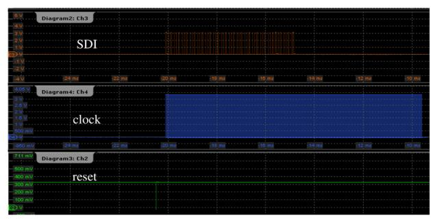
**Expected behaviour**: in this configuration, the BASIC32 acts as a shift register; during the first 524 clock cycles the input sequence is stored inside the register; at the 524th clock edge the input data begin to flow through the serial data output (SDO)
