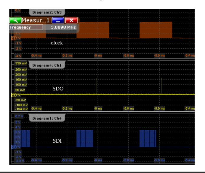
► Serial I/O test at 5 MHz: the system seems not working
