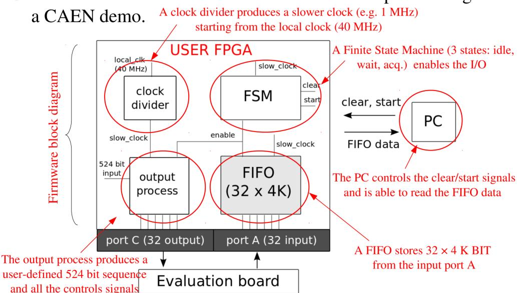
▶ During the first test, the serial data input (SDI) of the BASIC32 is driven with a 524 bits sequence and 1048 clock cycles.
