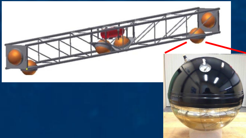
Large PMTs on tower structure (NEMO concept)
