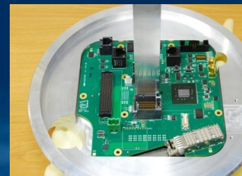
CLB (left) and power-board (right) in 'mushroom' structure
