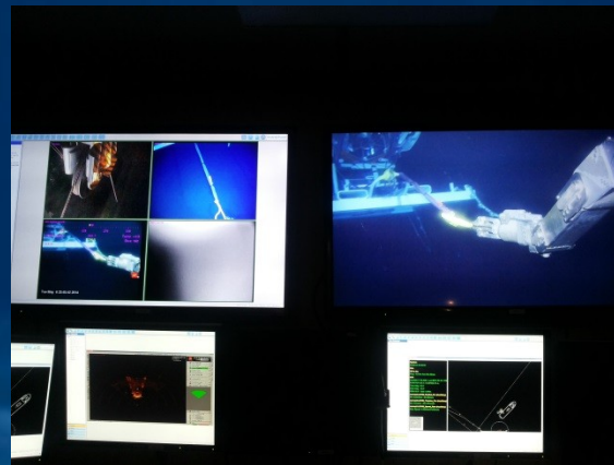
ROV orienting the anchor of the PPM-DU
