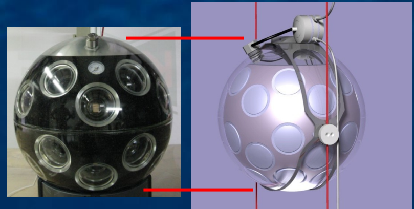
Multi-PMT DOMs (*) on string structure
